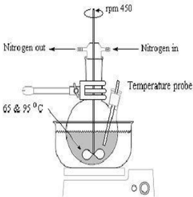
Figure 2: Reaction vessel for microsponge preparation by liquid-liquid suspension polymerization [26]
