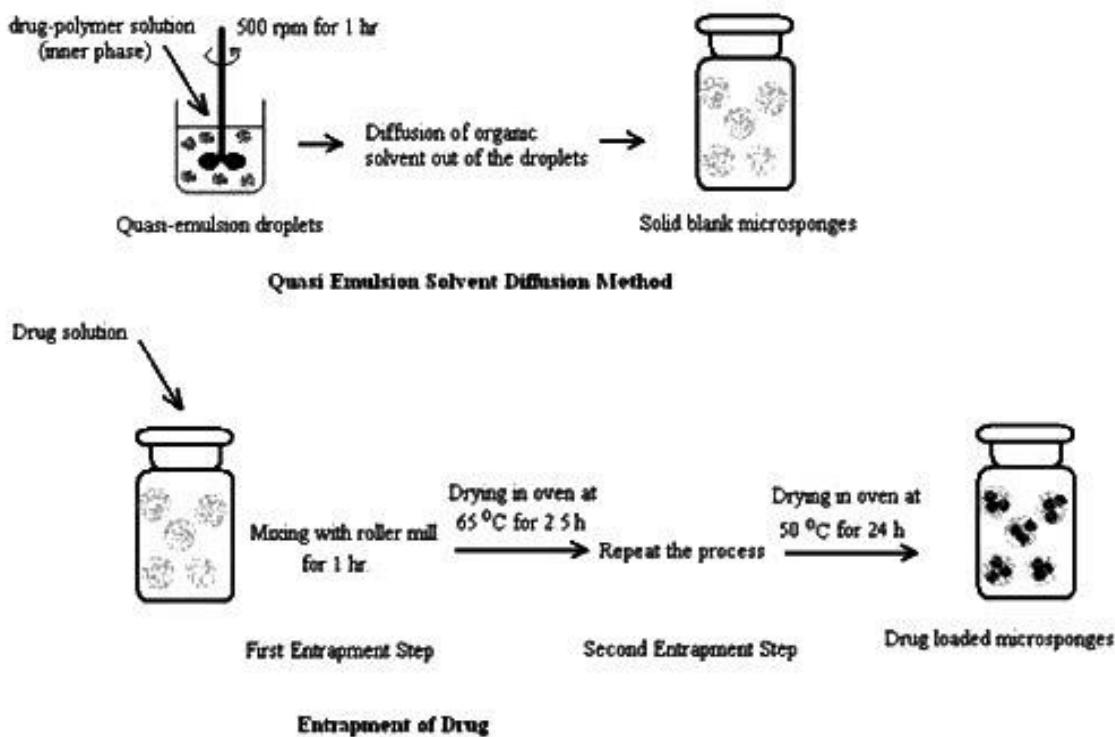
Fig 3: Preparation of Microsponges By Quasi-Emulsion Solvent Diffusion Method [28]
